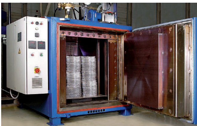
Anlassofen · Tempering furnace
